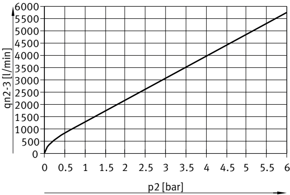
Flow rate qn from 2 -> 3 as a function of excess output pressure p2, VPPM-12L-...-0L6H-... (8 bar)
